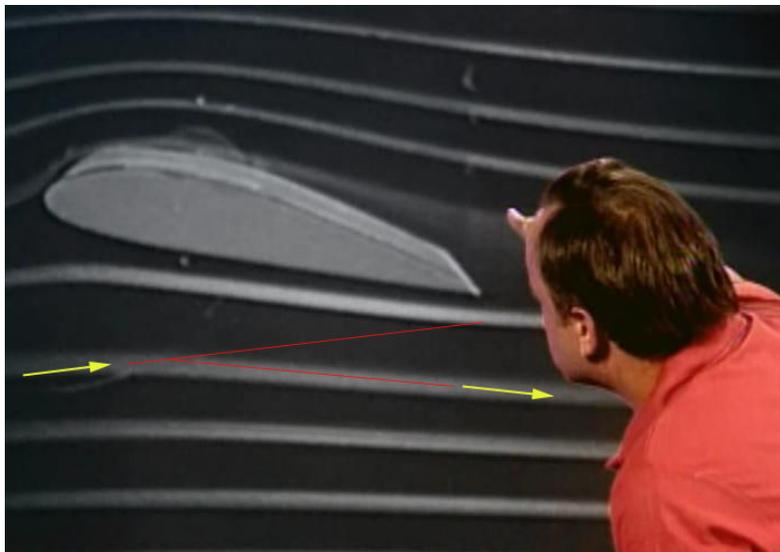
called *Downwash*. The answer to how the bulk of the lift is generated is latterly right under this guys nose, but he is pointing to the top of the wing. Experiments have shown that the overall downwash flow generates about most of the total wing lift.
